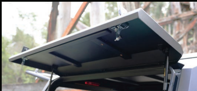
LARGE REINFORCED GULLWING DOORS WITH GAS ASSIST STRUTS FOR EASY OPENING AND CLOSING
